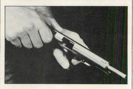
"Immediate action" malfunction drills start by ensuring the magazine is properly seated, and retracting the slide to eject the round or empty cartridge. Photo: Tom Slizewski
